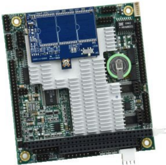
Helios with heat sink and flashdisk installed
