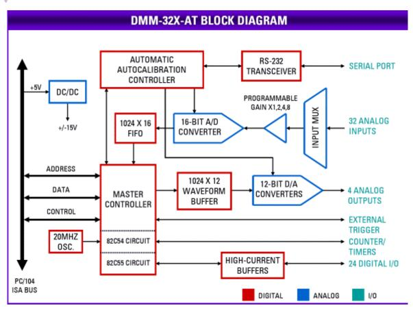
At the core of DMM-32DX-AT is an FPGA with advanced logic that provides important features needed to get the most out of your system:
