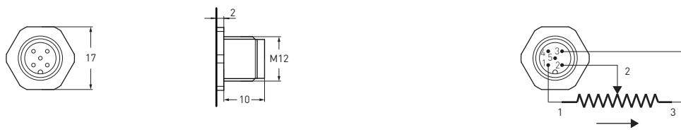
CN5A: 5 pin, M12 connector (optional)
