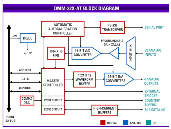
At the core of DMM-32X-AT is an FPGA with advanced logic that provides important features needed to get the most out of your system:
