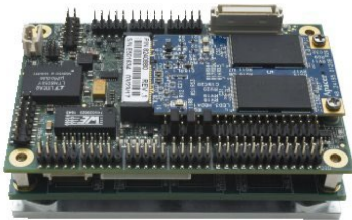
Zeta Carrier Board top, with data acquisition
