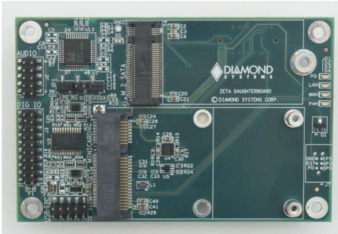
ZETA-DB-01 full-feature daughterboard with expansion sockets, audio and GPIO
