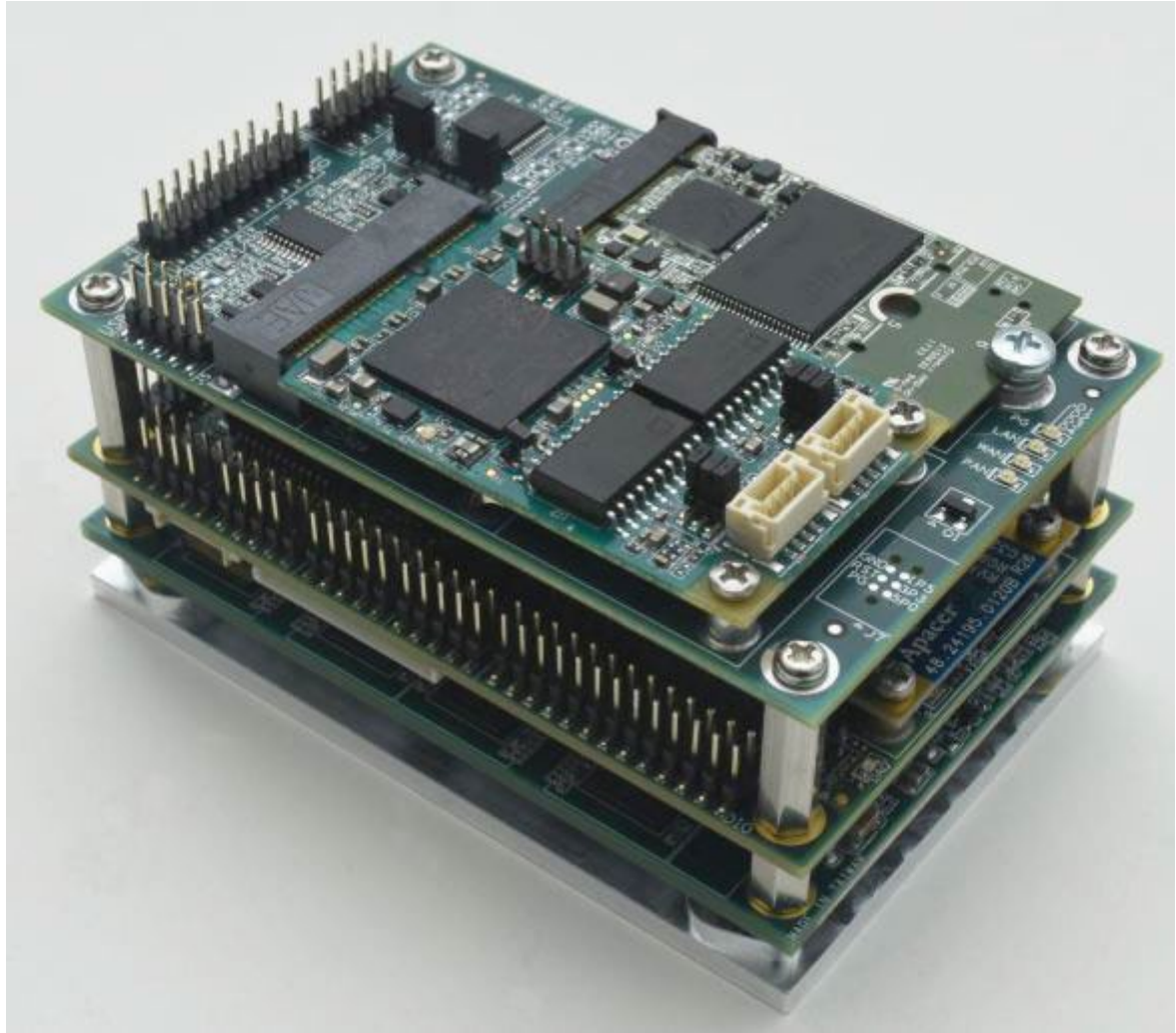
Zeta SBC with full-feature daughterboard and modules installed
