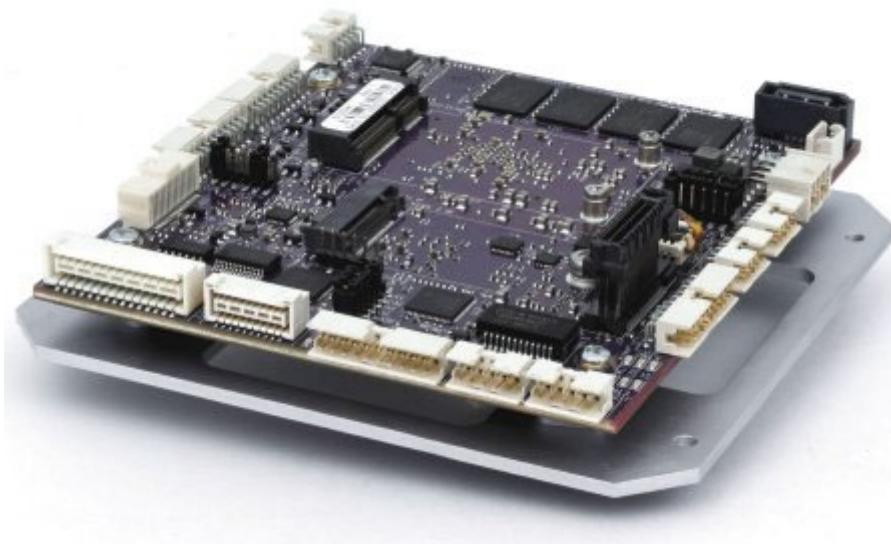
Edge view showing heat spreader and latching connectors
